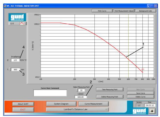
Fig. 3.10 Curve plotting
