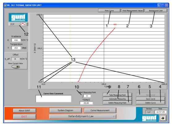
Fig. 3.8 Curve plotting screen
