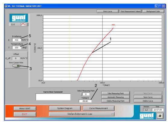
Fig. 3.14 Curve plotting
