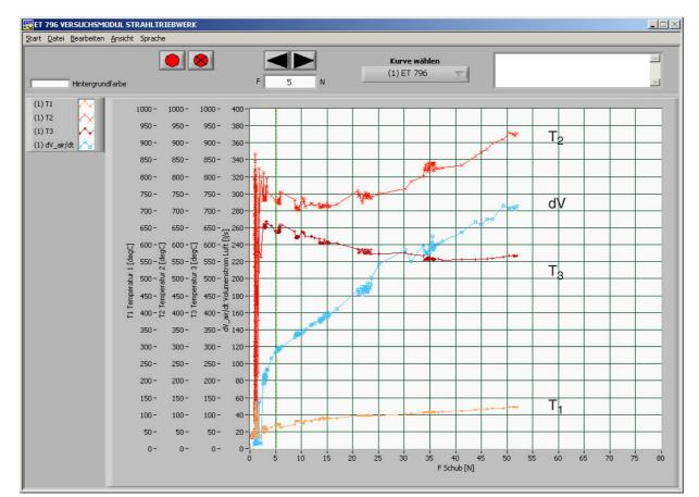
The following diagram shows the relation between air consumption, thrust and some temperatures.
