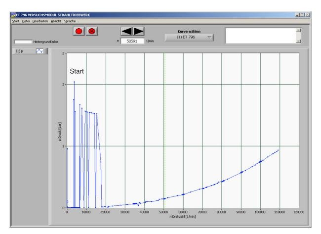
Fig. 5.5 Combustion chamber pressure of the jet turbine from start up to 120000 rpm.
