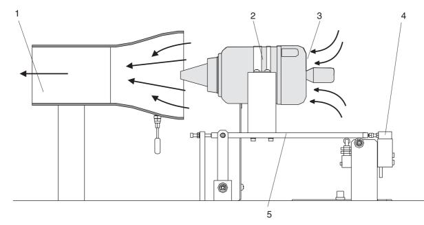
Fig. 2.4 Jet turbine with mixing tube and thrust measurement
