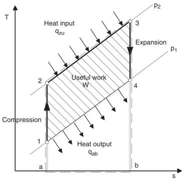
Fig. 4.2 T,s-diagram of gas turbine process
