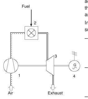
Fig. 4.1 Simple, open gas turbine system
