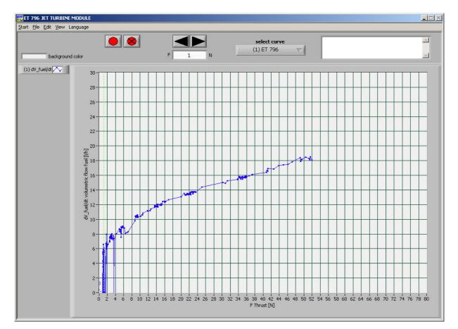
The following diagram shows the influence between fuel-consumption and thrust.
