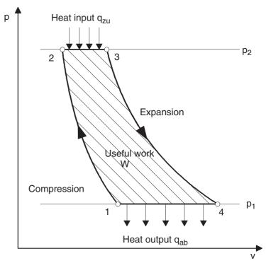
Fig. 4.3 p/v diagram of gas turbine process
