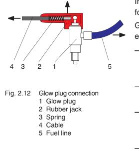
In case of starting problems, check the glow plug for damage or dirt clogging.
