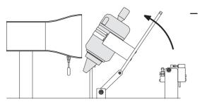
Fig. 2.11 Swivel turbine to remove residuel fuel
