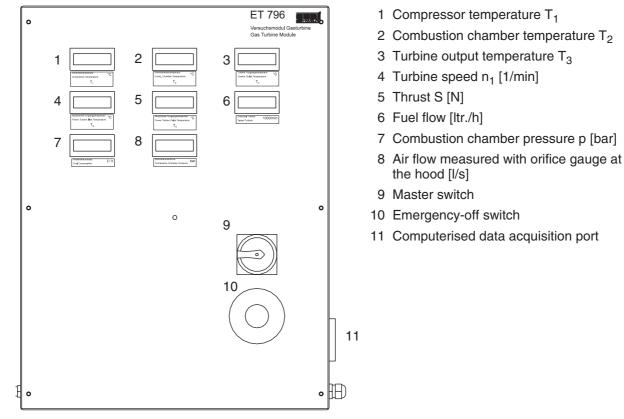
Fig. 2.5 Front panel with indicators
