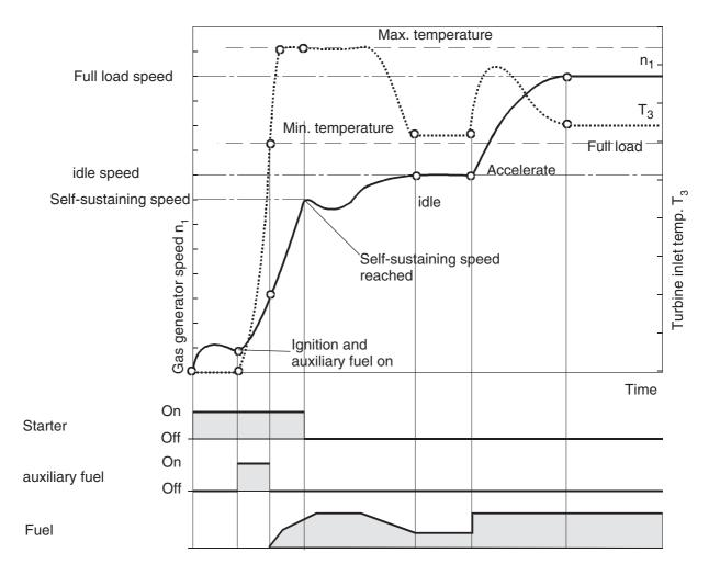
Fig. 2.10 Start-up procedure
