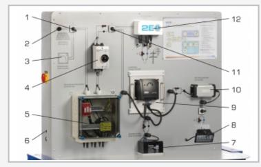
1 toggle switch: photovoltaic simulator/photovoltaic module, 2 photovoltaic module connection socket, 3 symbol for photovoltaic simulator, 4 DC switch-disconnector, 5 combiner box, 6 module temperature and illuminance connection socket, 7 solar battery (stand-alone), 8 lamp (stand-alone), 9 charge controller with MPP tracker (stand-alone), 10 inverter (stand-alone), 11 toggle switch: grid-connected/stand-alone, 12 inverter with MPP tracker (grid-connected)
